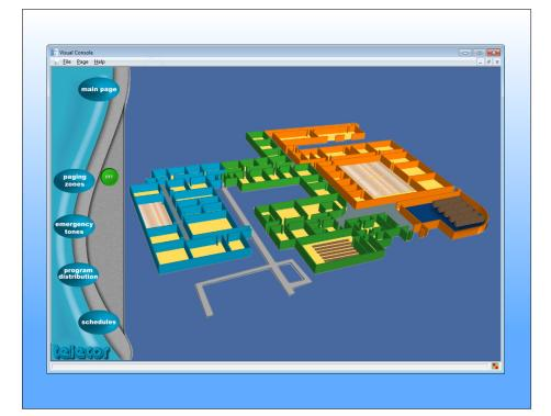
In Visual Console, you can create a Custom Operating Screen using a bitmap layout of the building as the background. Icons representing intercom stations, paging zones, and audio program zones are incorporated onto the floor plan.
