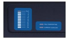
A calibrated LED level meter indicates the amount of signal present in 3 dB steps, from - 30 dB to -3 dB. The clip LED lights whenever the output stage is about to clip from either an overdriven input or an overloaded output.
