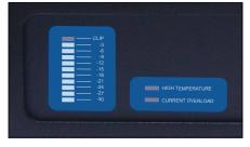
A calibrated LED level meter indicates the amount of signal present in 3 dB steps, from - 30 dB to -3 dB. The clip LED lights whenever the output stage is about to clip from either an overdriven input or an overloaded output.
