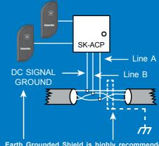
Earth Grounded Shield is highly recommended in environments subject to high voltage electrical discharge (ie. lightning). Shield should be connected to earth ground only at one end of the cable. DC Signal Ground may be necessary in networks with very long wire runs. DC Signal Ground wire is **NOT** to be connected to earth ground.
