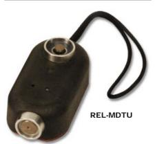
The Reliant Mobile Data Transfer Unit, with a capacity of 21,842 readings, can collect the data from several Reliant DAUs. This makes it unnecessary to take a portable PC to several sites or to bring the DAUs to a central location for downloading.
