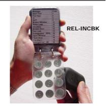
Incidents may be recorded using the Reliant Incident Book. Incidents are pre-defined and assigned numeric codes in the Reliant PLUS software. Incidents observed by the officer are recorded during a tour by entering the incident's code, using the touchmemory keypad.
