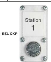
The Reliant checkpoints use stainlesssteel touch-memory iButtons. Each iButton has a unique 16-digit ID number that identifies the checkpoint, security officer, supervisor, etc. to which it is assigned. The iButtons are assembled into checkpoints using clear polycarbonate shells and mounted with the self-threading screws provided.
