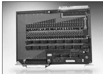
Contains the circuitry to control 25 remote LEDs. It tracks annunciate/output point activity and then produces a drive signal to light up the corresponding LED. Typical applications include Call Confirmation and Message Waiting LEDs found with Room Stations and Graphic Annunciators.
