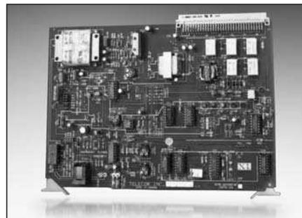
The PBI-6-MA is an interface card that allows DTMF telephones from a separate system to access the XL system and initiate intercom calls and paging announcements. The PBI-RG-MA is identical, but with the addition of a built-in 90-volt ring generator for Single Line Console integration.
